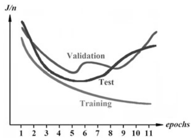
Fig. 6.19 A typical learning curve. The average error per pattern is plotted as a function of the number of epochs
