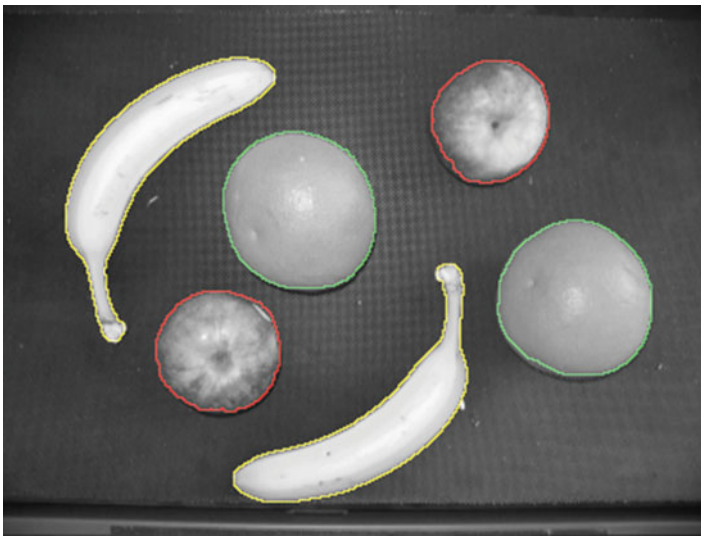
Fig. 2.16 Objects have been classified into three classes of fruit, and outlines superimposed on the original image
